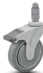
Our Directional Lock casters are designed to lock the swivel but not the wheel allowing you to steer your equipment. The directional lock feature is designed to break free under heavier load when the unit is traversing a corner only to lock back into position when the unit resumes a straight course.
