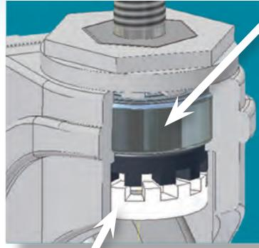
NG series has precision sealed ball bearing raceway design for long lasting, smooth, quiet, maintenance free ride. Precision ball bearings are insert molded into the swivel raceway. Caster capacity is similar to steel wheels at a massive 325 lbs with 5" wheel.
